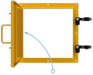
Benetech's Premium Plus & Premium doors include an optional deflector pan which creates a flat interior surface when the door is closed ensuring less dust accumulation on the frame.
